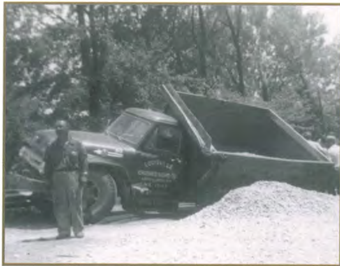
Safety is constantly discussed because accidents occur so easily. A shifting load caused this truck to overturn and lose its aggregate.
